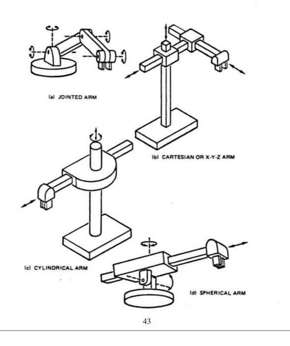
FIGURE 1 Four Common Arrangements of Robot Manipulator Joints
